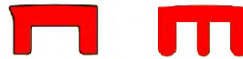
Lower magnet - available 9mm high, with 2 feet for exterior doors, and 3 feet for interior doors
